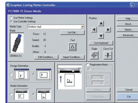
**Note:** If the Controller is launched from the Start menu, a [Close] button replaces the [Cancel] and [Cut] buttons.
